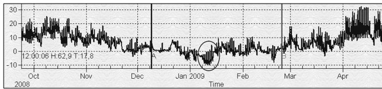
**Fig. 1** Temperature data from a storage building in Stuttgart/Germany recorded from October 2008 to April 2009 with an PCE-HT110 data logger showing temperatures down to  $-10^{\circ}\text{C}$  in January 2009
