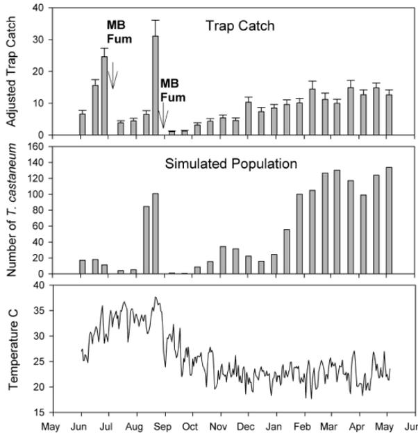
**Figure 2** Mean red flour beetle trap catch (2-week duration), model predicted insect numbers and hourly inside building temperatures for a flour mill located in central Kansas USA. The flour mill was fumigated with sulfuryl fluoride (111 g for 18 h) on 19 June 2004.
